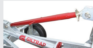
Adjustable top link to ensure stirrer is working at optimum depth.
